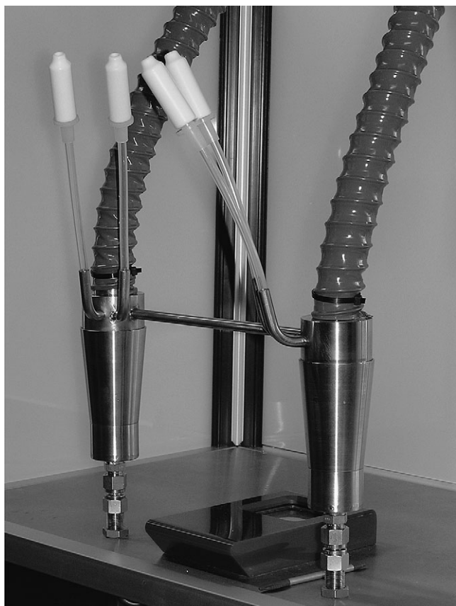
Figure 2 One set of sniffing ports. Each vessel terminates into 2 extensions with tightly fitting nosepieces to allow separate airstreams to each nostril. Odorized air bypasses the extensions to the exhaust and enters into the nose only during active sniffing (see text).
